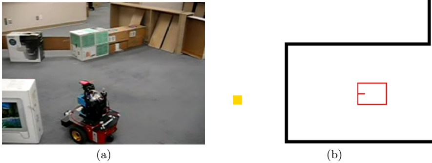
Fig. 3. Pioneer robot in the Real World (a) and VFH trap: The robot’s goal is to reach the small square outside the room (b)
